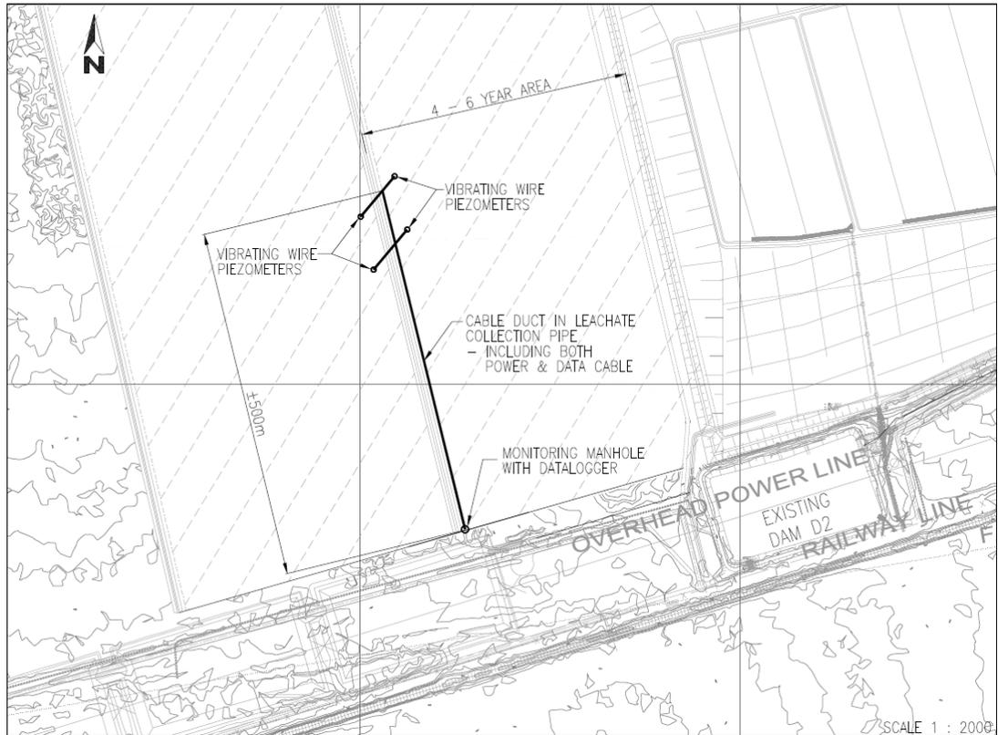
**Figure 3-10: Typical layout of temperature monitoring system**
