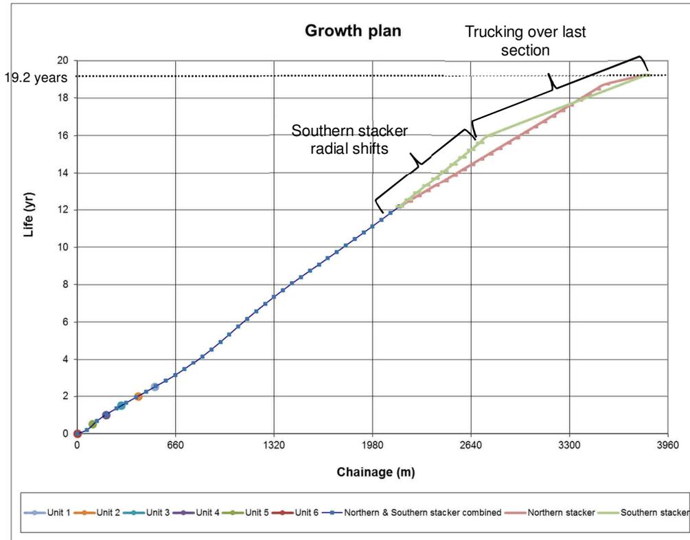
**Figure 8-1: Growth plan – Time vs. Chainage**
