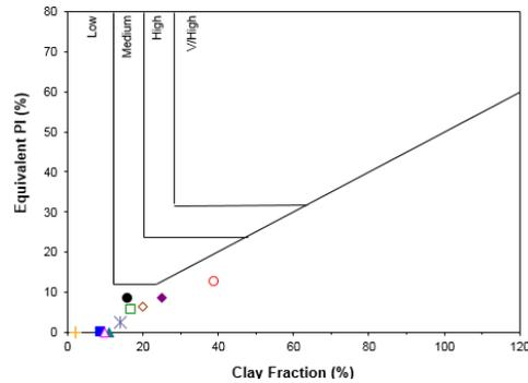
Figure 2-5: Grading Curves, Plasticity & Heaving Chart of the Material Tested
