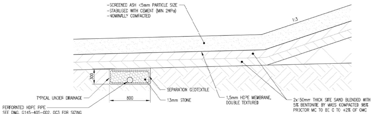
**Figure 3-8: Typical liner detail in PCDs**
