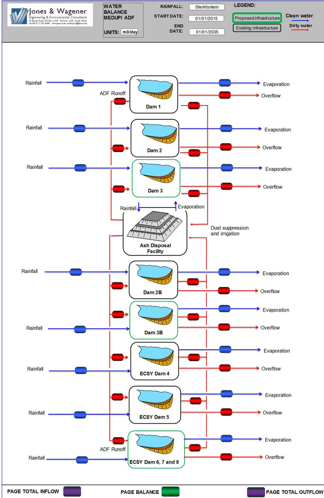
Figure 6-5: Schematic flow diagram for the Medupi NAGDF
