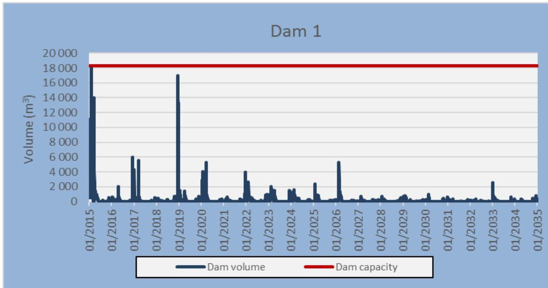
**Figure 6-6: Dam D1 dam volume over time plot**
