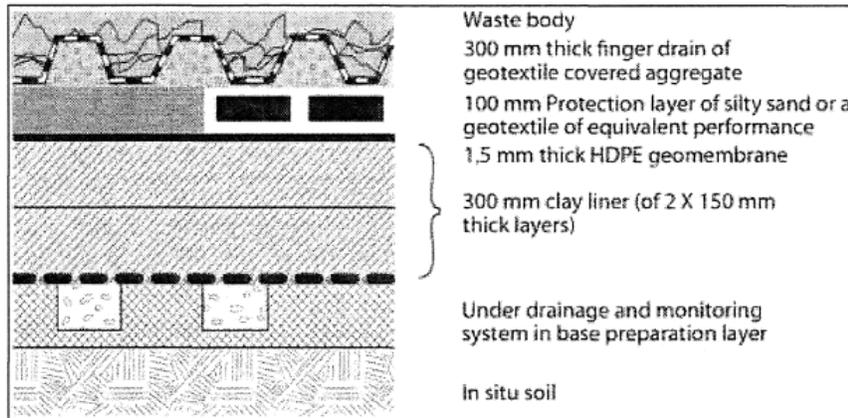
**Figure 3-6: Typical Class C Landfill barrier system**
